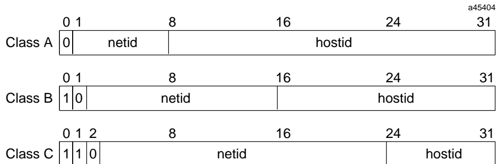
Figure C-1. IP Address Format for Network Classes A, B, C
