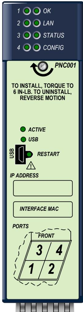
The PACSystems<sup>†</sup> RX3i PROFINET Controller (PNC) module, IC695PNC001, connects a PACSystems RX3i controller to a high-speed PROFINET local area network. It enables the RX3i controller to communicate with IO-Devices on the LAN. The PNC provides all the functions, services, and protocols required for certification as a PROFINET IO Version 2.2 IO Controller, running at both 100 Mbps and 1 Gbps.
