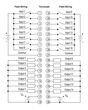
Inputs 1 to 16 form one isolated input group. Outputs 1 to 7 and 8 to 14 form two isolated output groups, each with its own voltage connections. Outputs should be evenly distributed between the two output groups, as discussed under "Output Points versus Temperature".
