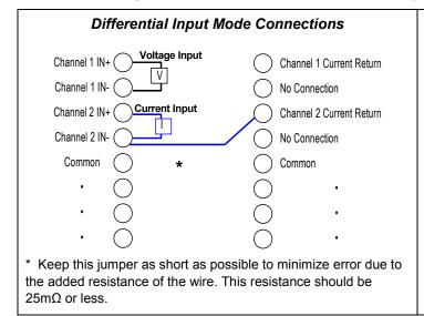
For differential inputs, two adjacent terminals are connected as one channel. The lower-numbered terminal acts as the high side.
