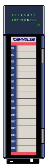
The **120/240VAC 16-Point Isolated Output** module, IC694MDL350, provides 16 individually-isolated output points. A high level of noise immunity minimizes the need for external snubbers to protect the outputs against transient electrical noise on the power line. The outputs can control a wide range of inductive and incandescent loads. Power to operate the output loads must be provided with an external AC power supply.
