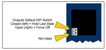
With the Outputs Default Mode switch in the right (open) position, the outputs will turn off whenever communication with the CPU is lost. When the switch is in the left position, the outputs will hold their last programmed value whenever communication with the CPU is lost.
