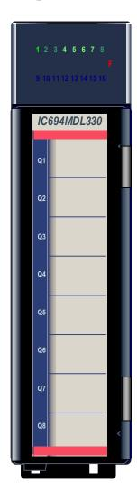
The **120/240volt, 2 Amp AC Output** module, IC694MDL330, provides eight output points in two isolated groups of four points. Each group has a separate common. The two commons are not tied together inside the module. The groups can be used on different phases of the AC supply or powered from the same supply. AC power to operate loads connected to outputs must be user supplied. This module requires an AC power source; *it cannot be used with a DC power source*.
