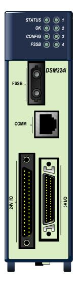
The DSM324 integrates high-performance motion control with the logic-solving functions of the RX3i PACSystem.
