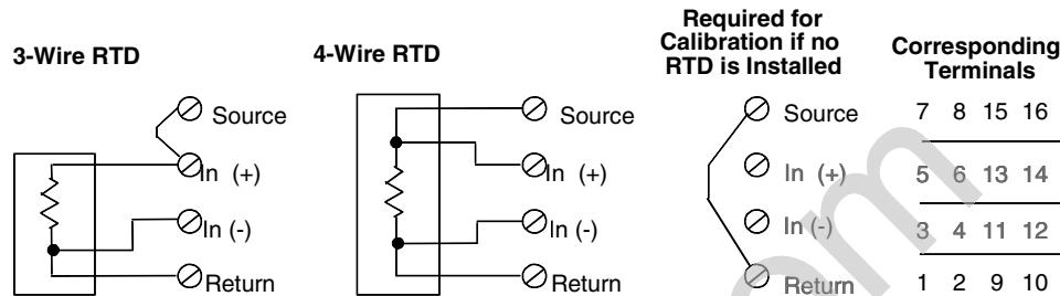
No loop power is required for this module. The excitation current for the RTDs is provided by the module, which automatically matches the excitation current to each configured RTD type.
