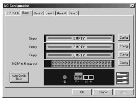
Figure 6.5 - Base 1 with an I/O Module Selected
