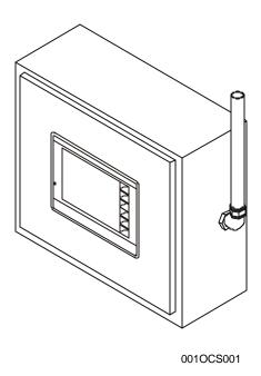
**NOTE:** There are <u>NO</u> orientation restrictions on the Color Touch OCS. However, the above orientation provides for <u>optimum readability</u> of the screen and <u>ease of use</u> of the keypad.
