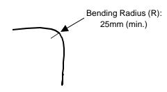
Figure 3.7 - Bend Radius (R) of Fiber Optic Cable
