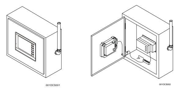
Figure 1.1 – Color Touch OCS (Shown in Panel Box)
