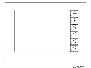
Figure 5.1 – Color Touch OCS Front Panel Keys
