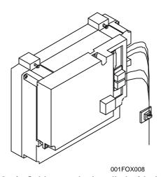
Note: Fiber Optic Cables can be bundled with the Power Cable.
