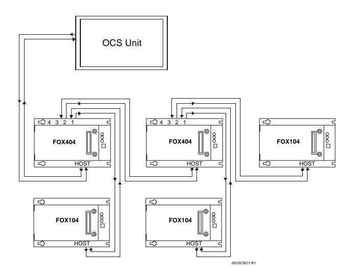
Figure 3.11 – Color Touch OCS to FOX (Multiple Hubs and Bases)
