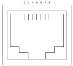
Figure 2.11 – Close-up of Port 1 /Port 2 (RS-232 and RS-485)
