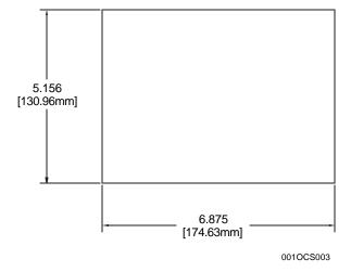
Figure 2.1 - Panel Cut-out and Dimensions
