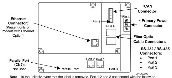
Figure 2.5 – Location of Ports and Connectors (Color Touch OCS with Ethernet Option Shown)
