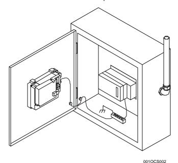
Figure 2.4 – Back view of Color Touch OCS (Shown On Panel Door)
