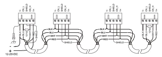
Figure 2.10 - CAN Wiring
