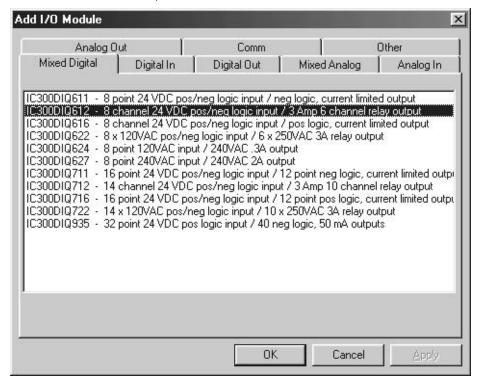
Figure 6.4 - Selecting an I/O Module
