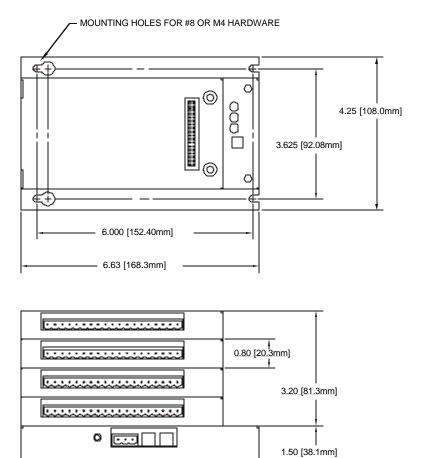
NOTE: Use #8-32 or M4 mounting hardware consisting of four pan head screws with external tooth lock washers.
