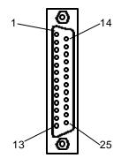
Figure 2.12 –RS-232 / RS-485 Connector (Port 3)
