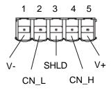
Figure 2.8 – Network Connector (CAN Port)
