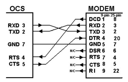
Figure 2.16 - Modem Wiring
