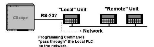
Figure 1.3 – Pass-Through Function (Available in CsCAN Networks Only)
