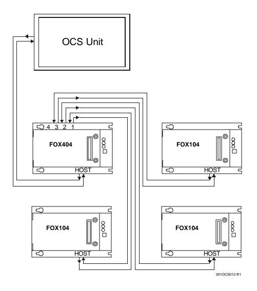
Figure 3.10 – Color Touch OCS to FOX (One Hub and Multiple Bases)
