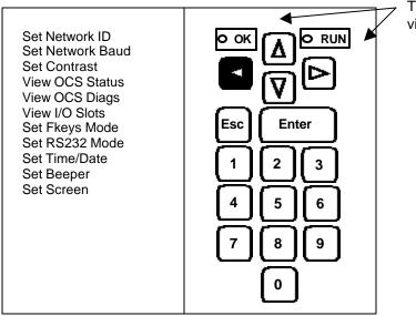
This screen is used to view Status LEDs.
