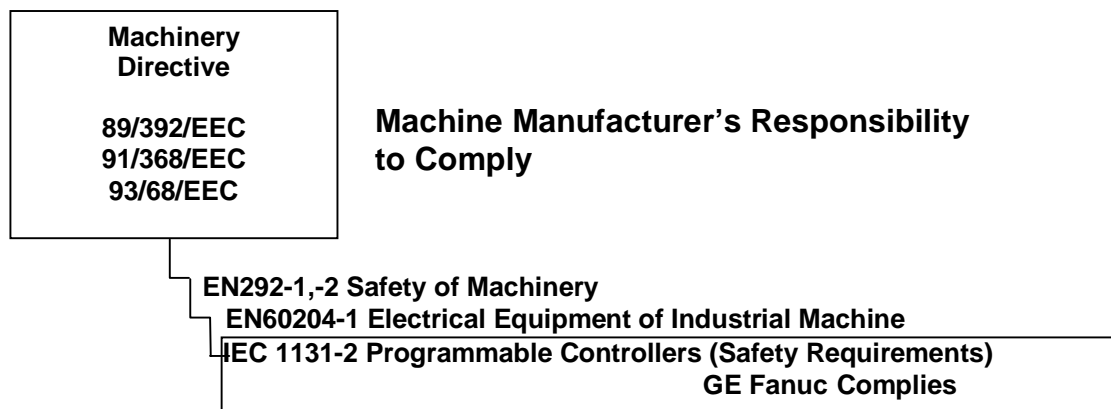
Figure 1-8 GE Fanuc's Path for Supporting Machine Manufacturer's Compliance with the Machinery Directive
