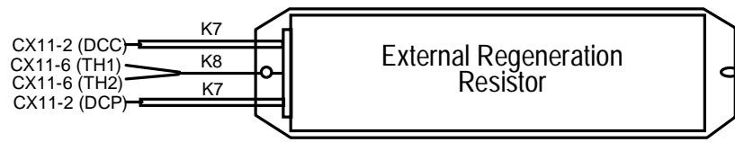
Figure 2-15. Connecting the External Regeneration Resistor
