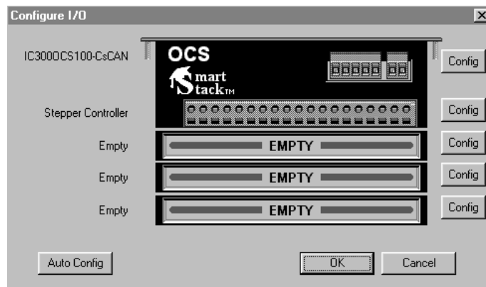
Figure 3.4 – STP100 Module is Added
