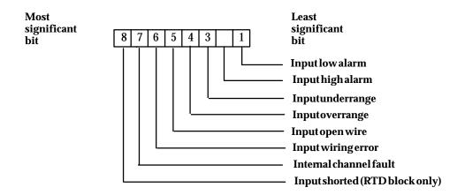
Analog output diagnostic bytes (AQ\_DIAG) for Genius analog blocks and Series 90-70 integral analog output modules contain the fault information shown in this table.
