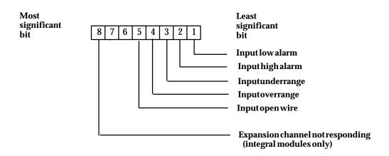
Analog input diagnostic bytes (AI\_DIAG) for Genius RTD and Thermocouple blocks contain the fault information shown in this table.
