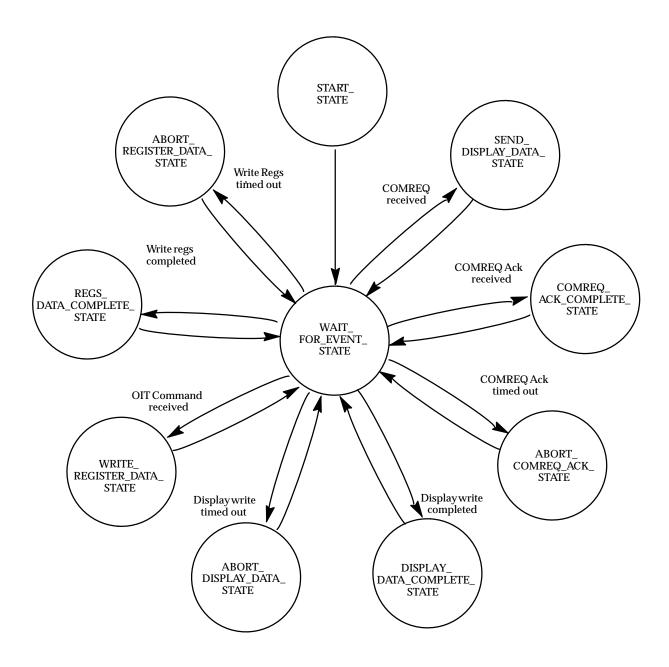
Figure 6.1 State Transition Diagram Of AST Based Example
