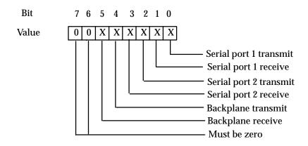
Combine the bits for the desired LED action into a single byte value in hexadecimal format. For example, to blink LED USER1 when characters are transmitted or received on serial port 2, use binary code 00001100. This is equivalent to 0C hexadecimal, so the command is:
