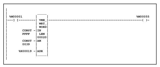
The PCM must be located in the rack and slot corresponding to the address contained in %R00019 and %R00020. The PCM C application would read this data from the PCM VMEbus dual port RAM by using, for example, a memcpy function call.
