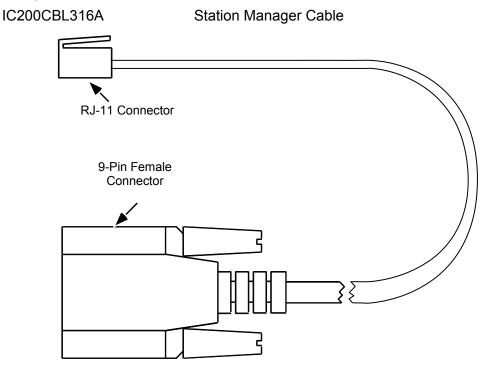
The end of the cable with the six-pin RJ-11 connector connects to the Station Manager port on the CPU372 *PLUS* or CPU374 *PLUS*. The end of the cable with the nine-pin D-type connector connects to the RS-232 serial port on your PC or terminal.
