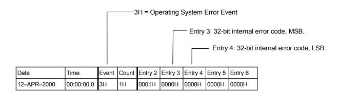
The table below shows the Operating System Error events and corresponding PLC Fault Table entries. Entry 2 identifies the particular Operating System Error event. Entries 3 and 4 contain a 32-bit internal error code. Entry 3 contains the most significant 16 bits; Entry 4 contains the least significant 16 bits. Entries 5 and 6 contain an internal location identification code.
