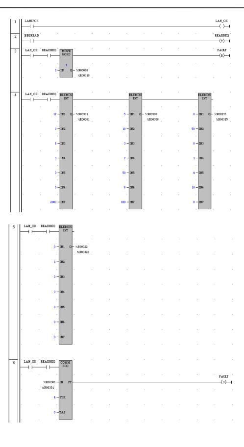
**Rung # 1**: Input LANIFOK (bit 16 of the LAN Interface Status bits) monitors the health of the Ethernet Interface. If it is OK to send a COMMREQ, the LAN\_OK coil is ON. LAN\_OK is used as an interlock for Rungs 3–6.
