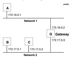
When host B with IP address 172.17.0.1 communicates with host C, it knows from C's IP address that C is on the same network. In an Ethernet environment, B can then resolve C's IP address to a MAC address (via ARP) and communicate with C directly.
