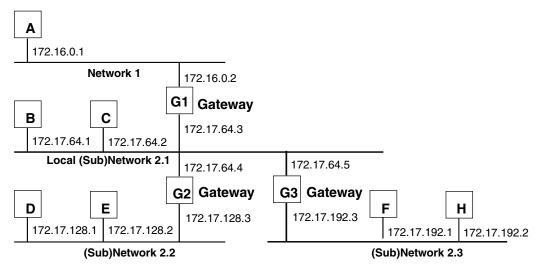
A PLC on Network1, Subnet 2.2, and Subnet 2.3 can talk to a PLC on one of the other networks without configuring multiple gateways because there is only one gateway on these networks. Gateway G1 would be configured as the default gateway for PLC A's Ethernet Interface; Gateway G2 for PLC D's and E's Ethernet Interface; and Gateway G3 for PLC F's and H's Ethernet Interface. The default gateway is configured in the Ethernet Interface's module configuration.
