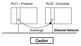
Ethernet Global Data is designed for simple, efficient communication of sampled data between devices. It is not intended for event notification where the possible loss of a sample of data would be significant. For event notification, it is recommended that an Establish Read/Write Channel command be used. See Chapter 3, "Programming SRTP Channel Commands", for more information.
