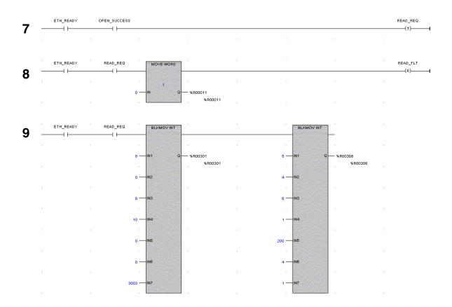
Rung #7: When OPEN\_SUCCESS is set it triggers READ\_REQ, which enables execution of the BLKMOV, MOVE and COMMREQ functions for the Modbus/TCP Read Commreq.
