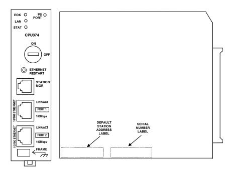
The Series 90-30 CPU374 has several user-accessible elements (only the Ethernet Interface's applicable elements are discussed here.)
