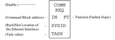
Each of the inputs and outputs are discussed in detail below. It is important to understand that the Command Block address points to the location in memory you have setup as the Command Block.
