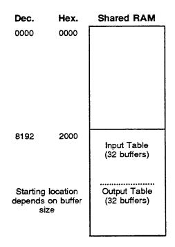
The Input Table contains inputs and incoming Global Data. GENI automatically updates the Input Table with new inputs every bus scan unless I/O Lockout is enabled.
