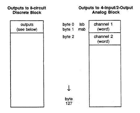
Discrete outputs are stored as individual bits, so outputs from an 8-circuit discrete block are stored in 1 byte of the Output Table (regardless of the block's actual I/O usage).
