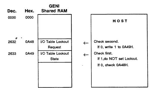
GENI automatically reads the state of the Lockout Request byte. GENI will not permit lockout while it is in the process of writing inputs or reading outputs in the I/O Table. After completing any I/O Table access currently in progress, GENI will set or clear the Lockout State byte to match the content of the Lockout Request byte.
