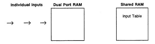
Unless I/O Lockout is enabled, GENI moves all the inputs in Dual Port RAM to the Shared RAM Input Table once per bus scan.
