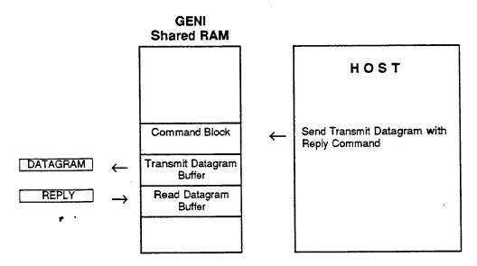
A datagram that generates a reply cannot be broadcast; it must be directed to a specific device on the bus. It can be sent with either normal priority or high priority. See "Transmit Datagram" for information about datagram priority.
