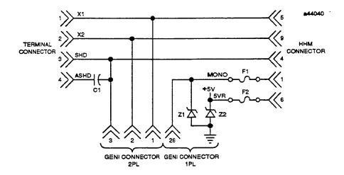
X1, X2, SHD, and AUXSHD must be 1/16 inch from all other signals on the motherboard. MONO and 5VR must be 1/16 inch from all other signals on the motherboard up to the high voltage suppressors, at which point, they may be grouped with the other motherboard 5 volt signals.
