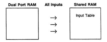
Input data is placed into the Input Table buffer associated with each device. That is, inputs from the device with Device Number 12 are placed in buffer 12.
