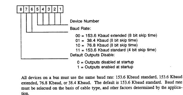
Device Number Each device connected to the Genius bus must have a unique Device Number assigned. This number represents the module's "bus address". The default Device Number set with the DIP switches on the GENI module is 31.
