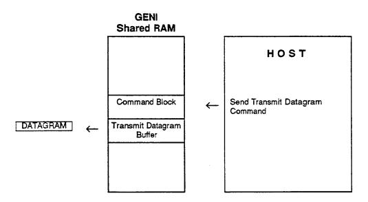
The datagram can be broadcast to all devices on the bus, or directed to a specific device.
