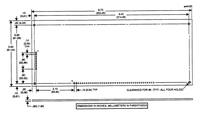
Connections to the motherboard are made by pins through the GENI board into a 10-pin connector and a 40-pin connector. The transformer and hybrid are located near the 10-pin connector to keep on-board electrical noise to a minimum.
