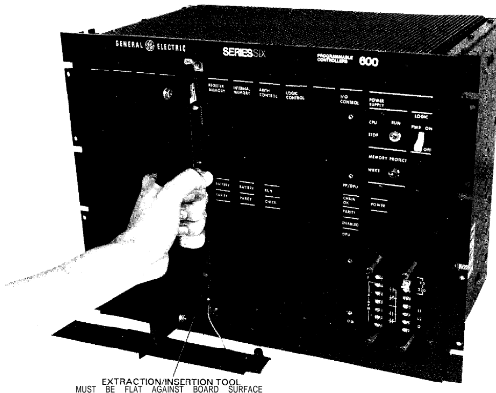
Figure 4. POSITIONING THE EXTRACTION/INSERTION TOOL FOR BOARD REMOVAL
