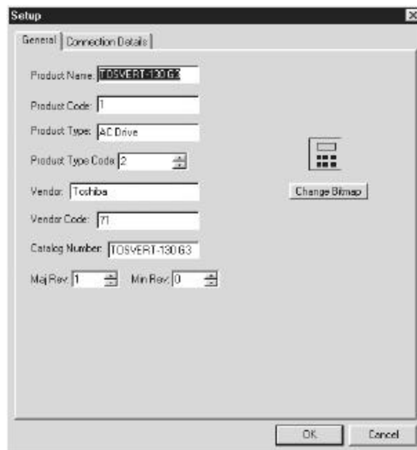
Figure 6.3 – Setup Screen in an EDS File (General Tab Selected)
