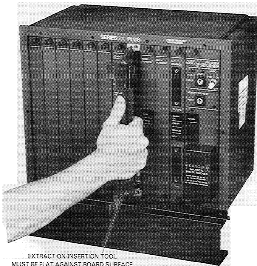
Figure 3.5 POSITIONING THE EXTRACTION/INSERTION TOOL FOR BOARD REMOVAL
