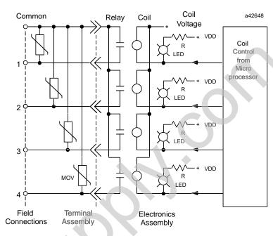
**NOTE:** Relay Normally-Open version shown. Normally-closed is the same, except for relay type.
