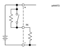
For a 24/48 VDC block, the resistor should be 5.1K ohms, 1/2 Watt or larger. For a 24 VDC block, the resistor should be 1.6K ohms.
