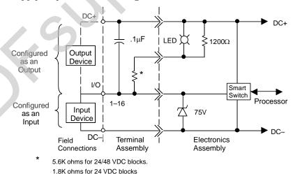
For 24/48 Volt DC Blocks, the internal resistor is 5.6K ohms. For 24 Volt DC blocks, the internal resistor is 1.8K ohms.
