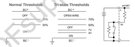
With the switch closed (ON state), the circuit senses the low source impedance. With the switch open (OFF state), the circuit senses the added resistance. If a wire is broken, cut or removed, impedance becomes very high. The block will transmit 0 as the state of the input, and send an OPEN WIRE message.
