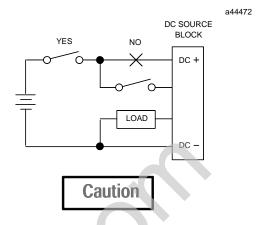
If circuit power is not removed at the same time as block power, the block may power up when multiple inputs are activated, even though one leg of power has been removed from the block.
