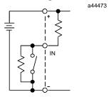
For a 24/48 VDC block, the resistor should be 5.1K ohms, 1/2 Watt or larger. For a 24 VDC block, the resistor should be 1.6K ohms.
