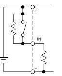
For a 24/48 VDC block, the resistor should be 5.1K ohms, 1/2 Watt or larger. For a 24 VDC block, the resistor should be 1.6K ohms.
