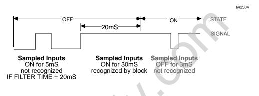
An input filter helps reject spurious noise spikes and multiple inputs generated by the bounce of mechanical devices. In controlled, noise-free environments, signals generated by clean, solid state electronics may be unnecessarily slowed by a filter, delaying system response. In such an environment, no additional filter time is needed.
