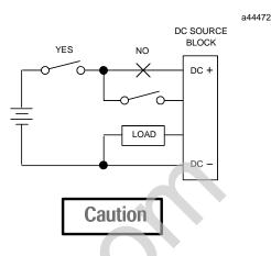
If circuit power is not removed at the same time as block power, the block may power up when multiple inputs are activated, even though one leg of power has been removed from the block.
