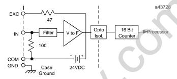
Each input circuit has a 24 volt current loop power supply, capable of providing 25mA of current. Each input is isolated from all other circuits on the block. Input accuracy is 0.1%. Input conversion time can be selected to provide the appropriate combination of noise rejection and input resolution. Conversion times are programmable from 16mS to 400mS. Resolution increases as the conversion time is lengthened. Input resolution is  $1\mu A$  for 200mS conversion time.
