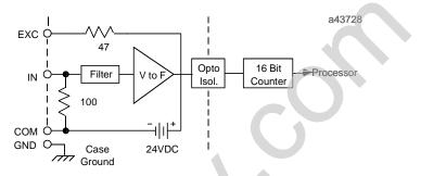
Each input circuit has a 24 volt current loop power supply, capable of providing 25mA of current. Each input is isolated from all other circuits on the block. Input accuracy is 0.1%. Input conversion time can be selected to provide the appropriate combination of noise rejection and input resolution. Conversion times are programmable from 16mS to 400mS. Resolution increases as the conversion time is lengthened. Input resolution is  $1\mu$ A for 200mS conversion time.
